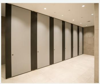
The cubicle partitions and pilasters were fixed to the floor and ceiling with fixing blocks for style and rigidity in equal measure. Meanwhile, the ceiling to floor cubicles and 20mm door clearances would guarantee total user privacy.
